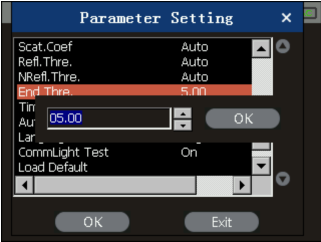
Figure 3-17 Setting the end threshold
