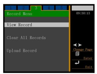
Press to enter "View Record" Menu, and press "**4**", "**>**" to select and view the Fusion-Splicing Records. Under this menu, it is possible to view the Fusion-Splicing Records for operating 6000-times.
