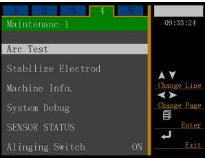
Press " $\blacktriangle$ " " $\blacktriangledown$ " to move the cursor, press  $\blacksquare$  to enter the program that you desire to get into, press " $\blacktriangle$ " " $\blacktriangledown$ " " $\blacktriangledown$ " " $\blacktriangledown$ " " $\blacktriangledown$ " " $\blacksquare$ " to modify the parameter values(via moving the cursor in the small pane); and press the key  $\blacksquare$  to confirm, so that the modification has completed. Then, press  $\blacksquare$  to quit.
