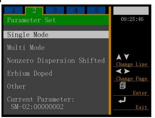
Press " $\blacktriangle$ " " $\checkmark$ " to move the cursor, and press  $\blacksquare$  to enter the "Fusion Splicing Mode" program that you want to get into.
