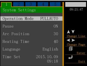
Press the keys " $\blacktriangle$ ", " $\blacktriangledown$ " to move the cursor; press the key  $\blacksquare$  to enter the program that you want to get into; press again the keys " $\blacktriangle$ "" $\blacktriangledown$ " " $\blacktriangledown$ " to modify the parameter values (via moving the cursor in the small pane); and press the key  $\blacksquare$  to confirm, so that the modification has completed.
